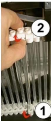
4. Remove the top pipette holder/pipette valve assembly (A) with a twist and pull movement. **NOTE:** The pipette valve assembly will sit inside the top pipette holder.
