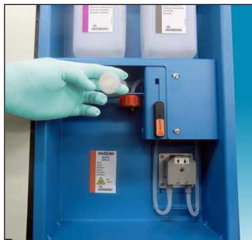
6. Replace the waste pump tubing by squeezing either side of the housing unit to release and gain access to the tubing.
