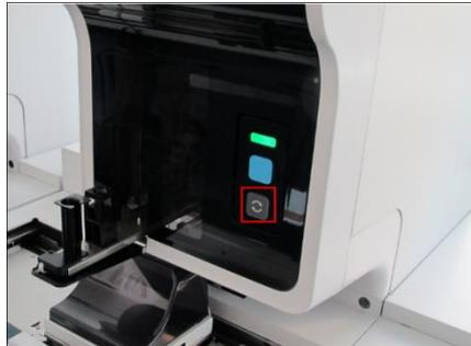
2. Once the manual tube holder has been ejected the [Change Analysis mode button] will appear on the IPU in the corresponding analyser menu.
