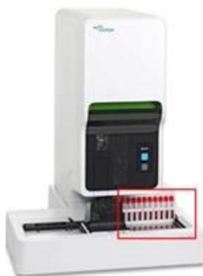
2. When processing is complete the rack will become available on the left hand side of the sampler unit.
