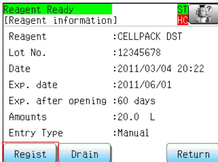
3. Enter the reagent information either by scanning the reagent barcode or by inputting the information manually.
