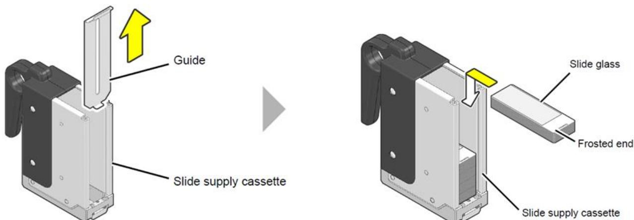
3. Replace the slide supply cassette guide, load the slide cassettes back into the slide supply unit and close the slide unit cover.
