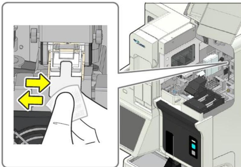
7. Once the clean is complete, restore all components back to their original position. On the IPU select [OK] to complete task.
