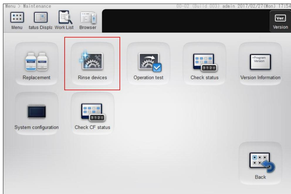
3. The [Rinse device] dialog box will appear. Make sure the smear unit cover is closed and Select [Spreader glass rinsing] followed by [OK]. The smear unit will now move towards the front to an accessible position.
