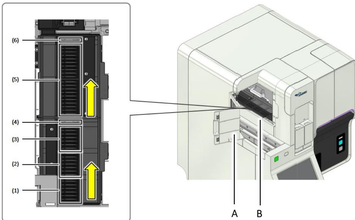
**A. Stain Unit Cover** – Open this cover to inspect the interior of the stain unit. Access can be gained for cleaning or maintenance tasks. Locked during operation.
