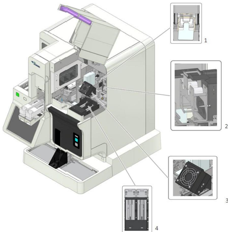
1. **Smear Unit** – Spreads the dispensed sample onto glass slide. Contains spreader glass unit.
