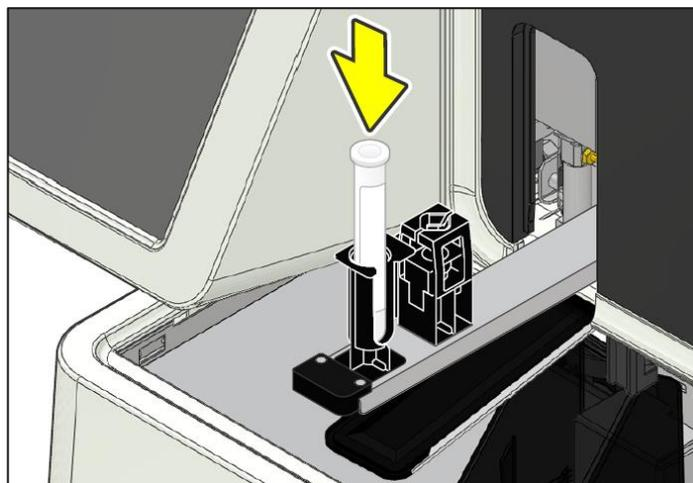
4. Press the Manual Analysis Start Switch. The sample tube holder retracts into the analyser and aspiration begins.
