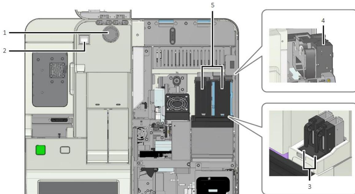
1. **0.07 MPa Regulator** – Regulates the source pressure to 0.07 MPa
