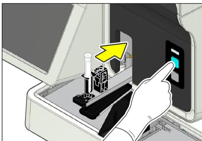
5. Shutdown 2 takes approximately 30 minutes depending upon the settings. The sample holder will eject forward once the CELLCLEAN AUTO aspiration finishes. Remove and discard CELLCLEAN AUTO tube once the sample holder ejects the empty tube. When all operations are finished, the sample holder automatically retracts into the main unit and the instrument shuts down.
