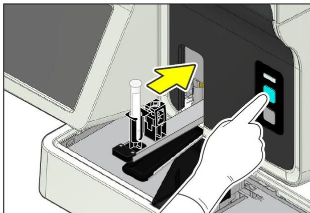
5. Shutdown 1 takes approximately 30 minutes depending upon the settings. The sample holder will eject forward once the CELLCLEAN AUTO aspiration finishes. Remove and discard CELLCLEAN AUTO tube once the sample holder ejects the empty tube. When all operations are finished, the sample holder automatically retracts into the main unit and the instrument shuts down.
