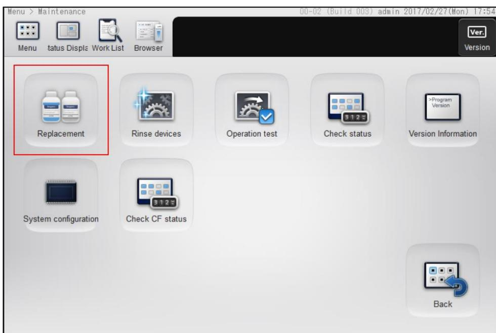
3. The [Replacement] dialog box will appear. Make sure the smear unit cover is closed and select [Replace spreader glass]. The smear unit will now move towards the front to an accessible position.
