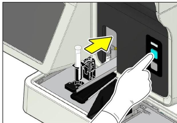
Once complete, remove sample and close the sample tube holder by pressing the mode switch on the front of the main unit.
