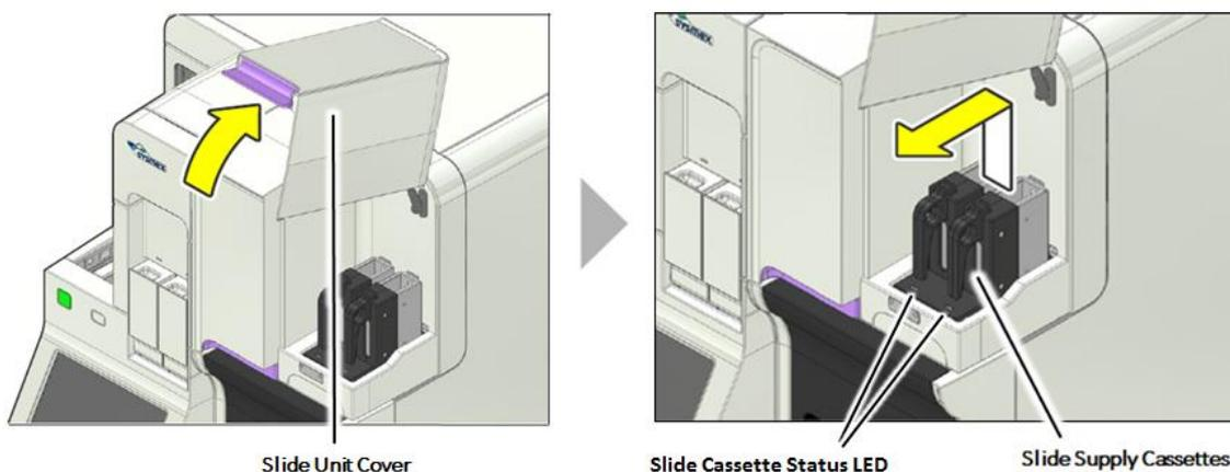
2. Remove the slide supply cassette guide and load in the new slides. Load the glass slides so that the frosted end faces upwards and is positioned toward the 'guide end' of the cassette, opposite end to the handle.
