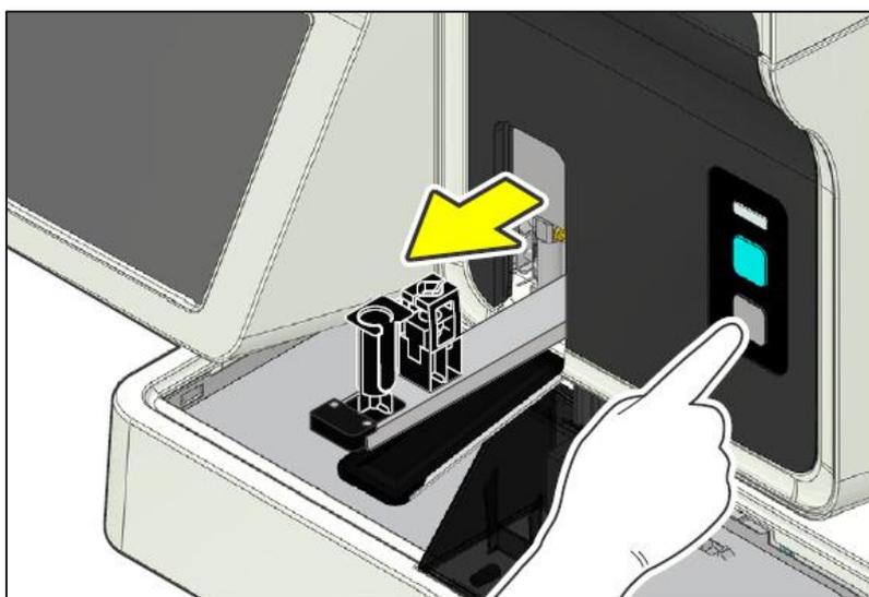
2. Check the status indicator LED of the instrument and magazine holders are **green**. Load an empty magazine into the manual magazine holder.
