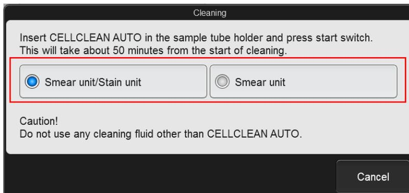
4. Follow the instructions on the IPU - Place 4mL CELLCLEN AUTO into the tube holder (cap removed).
