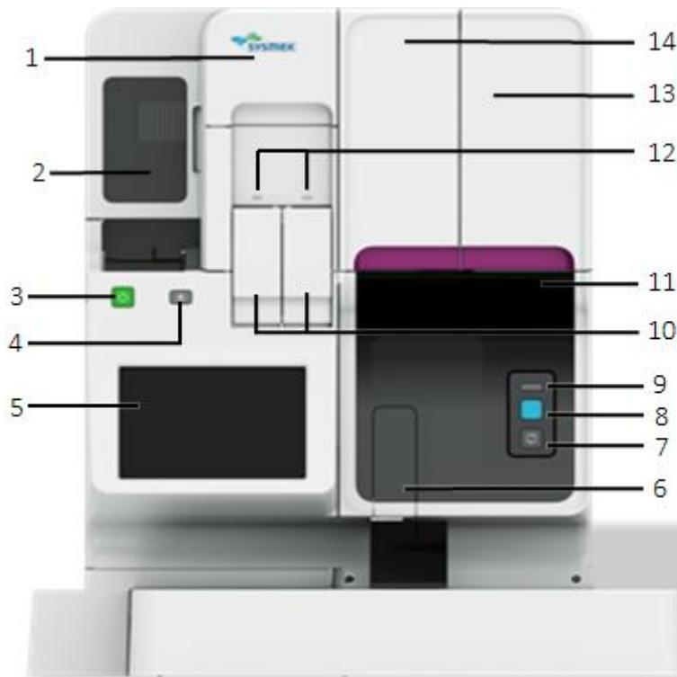
1. **Main Power Switch Cover** – Open this cover to turn the main power switch ON/OFF, and to regulate the pressures if required.
