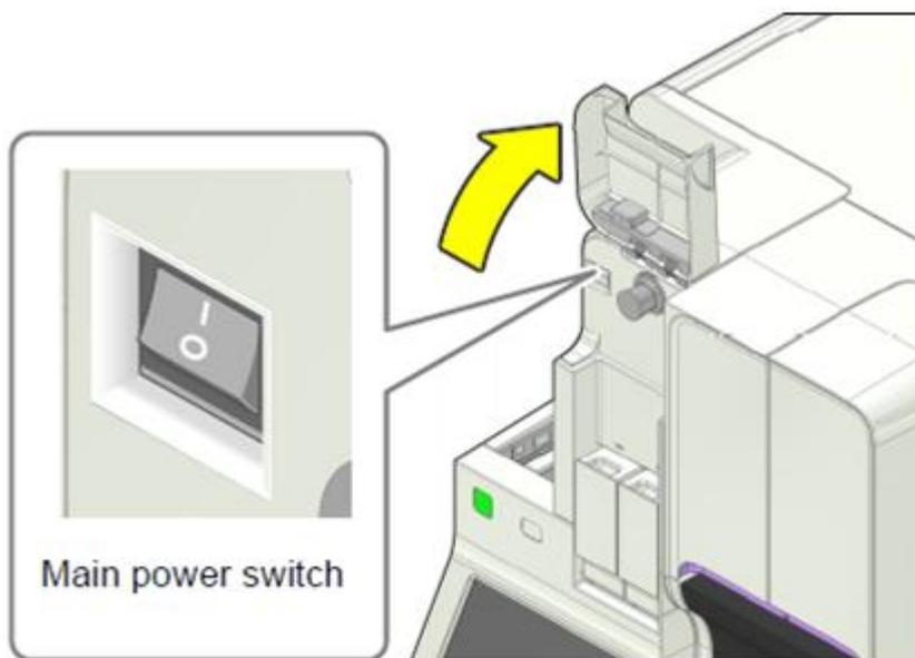
2. Press the start-up power switch to start up the instrument.
