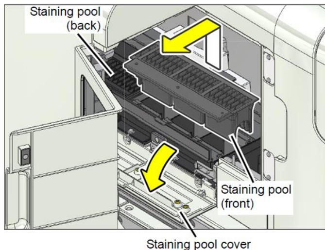
4. Clean the staining pool by soaking it in a rinse solution (Methanol, ethanol or lukewarm water). Make sure the staining pool is completely dry before placing back into the analyser.
