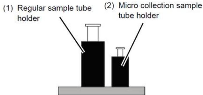
Press the start switch on the front of the main unit. The sample holder will retract and smear preparation starts. When the sample aspiration is completed the sample holder is ejected out automatically.
