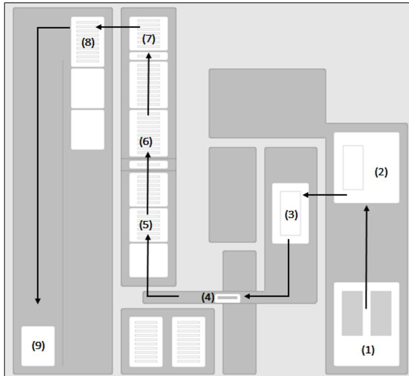
1. Once the barcode has been read the first step in smear production is for a slide to be removed from either slide supply cassette (1).
