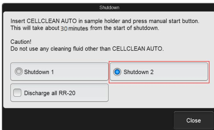
3. Follow the instructions on the IPU - Place 4mL CELLCLEN AUTO into the tube holder (cap removed).
