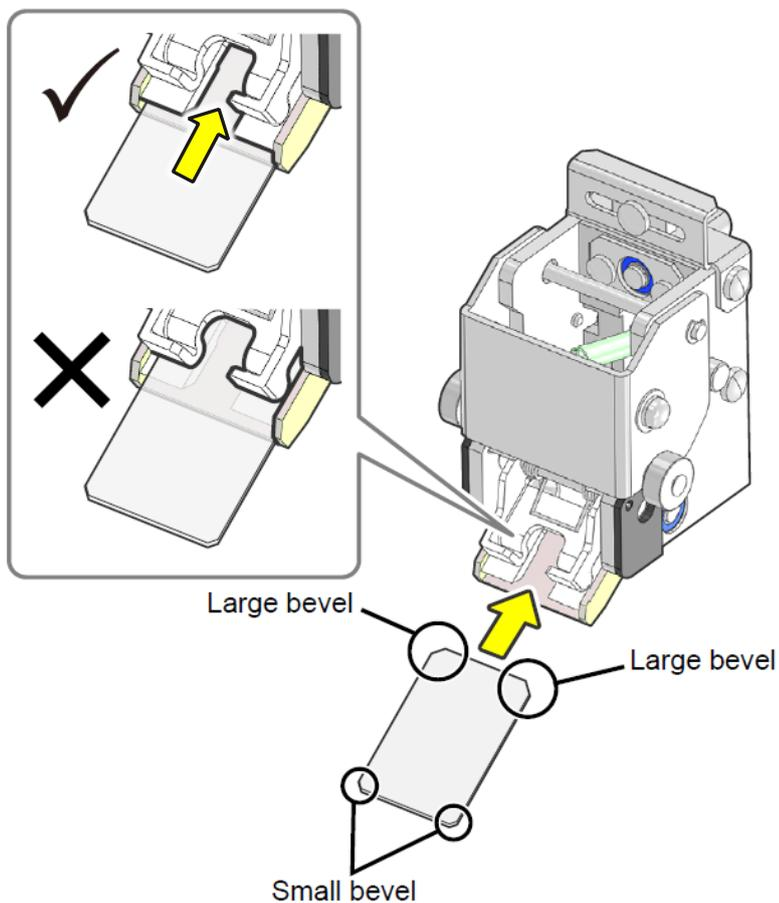
8. Once the spreader glass has been replaced, restore all affected components back to their original position. On the IPU, select [OK] on the spreader glass operation count followed by [OK]. This will reset the counter.
