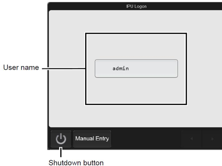
4. Once logged on the analyser will perform a self-check. This is to determine if there are any errors on the analyser. The self-check takes approximately 20 minutes and performs the following tasks:
