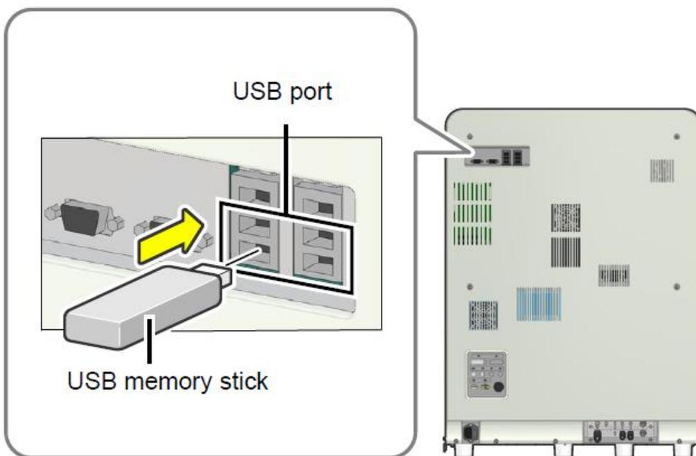
4. Select [File] from the top toolbar and select [Output in CSV Format]. The save starts and the [Waiting for completion] dialog box appears. When the dialog box closes, the save is complete. When performing a save, the file location/folder/name is automatically created on the memory stick.
