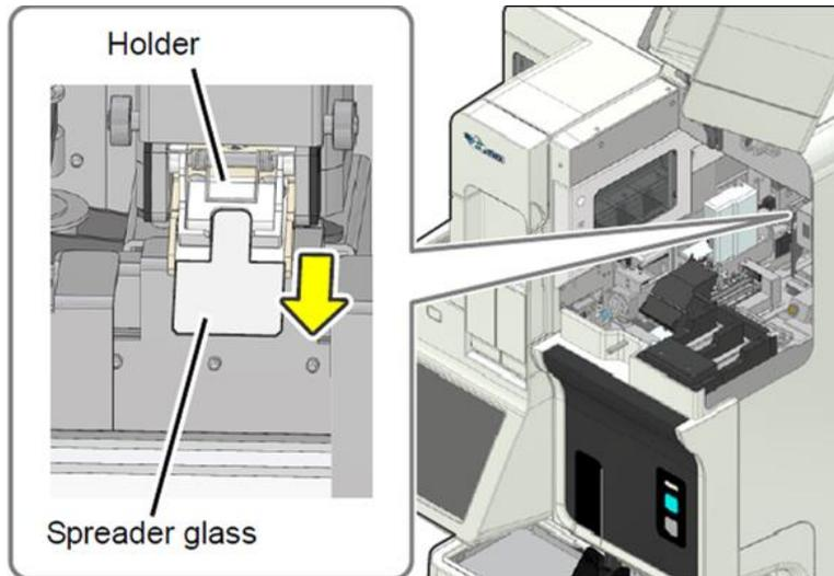
7. Set the new spreader glass in the holder. Set the spreader glass so that the edge with the small beveled edges faces forward. Insert the spreader glass all the way into the spreader glass holder until it stops.
