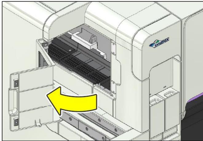
3. Pull the staining pool cover down and lift and remove the staining pools. Remove both pools, front & back.
