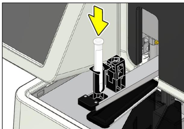
5. Press the Manual Analysis Start Switch. The sample tube holder retracts into the analyser and aspiration begins. When finished the holder is ejected forwards and the empty tube can be removed.
