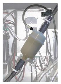
The bacterial filter needs to be replaced approximately every three months to prevent bacterial contamination of diluted reagent. When the filter needs changing the following error will be displayed on LCD screen 'Slow circulation error'.
