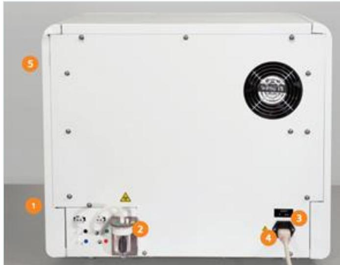
1. **Reaction Tube Trash Box** – Collects used reaction tubes and can hold up to 60 tubes, approximately.
