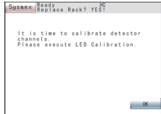
Press [OK] key, and follow the steps below to complete the LED Calibration
