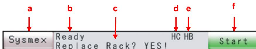
a. **Systemex Key** – Displays error list, temperatures and paper feed.
