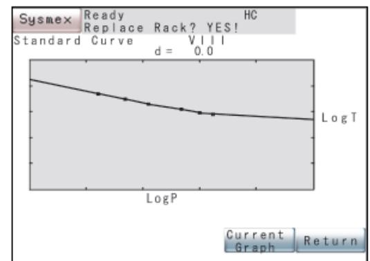
**Note:** When running PT- Multi Calibrator; if the dFbg method is also used on the instrument, the Derived Fibrinogen method must be disabled during the calibration with PT-Multi Calibrator to avoid overwriting the Derived Fibrinogen master curve.
